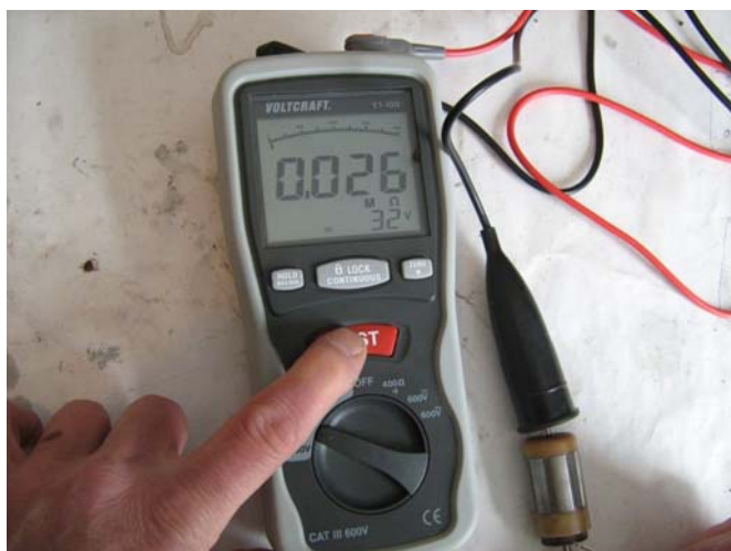
Pump armature being tested on the bench, the windings' insulation broke down at 32V.
